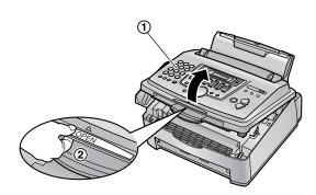
8 Install the drum and toner unit (1) by holding the tabs.
